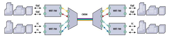
Where extended reach is required, the WRT-780 can be combined with WaveReady DWDM amplifiers and dispersion compensation modules to provide a dense and compact DWDM transport solution.
