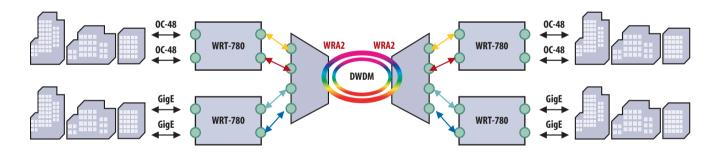
With the growing need to have storage area networks (SANs) extended over long distances to support enterprise connectivity or disaster and recovery solutions, the WRT-780 can be combined with the WaveReady WDM platform to offer a simple, reliable, and cost-effective SAN transport solution.
